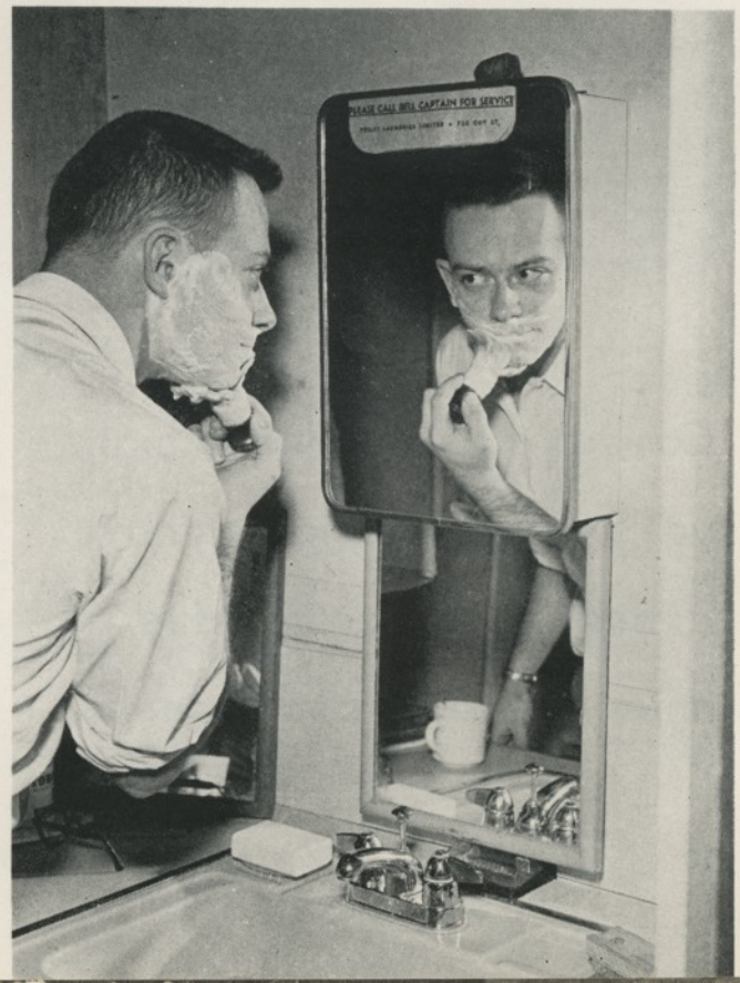
Here Bateman shaves in the car's bathroom, formerly generator room, in which completely up-to-date fixtures have been installed. Water is pumped automatically from a nearby well.
