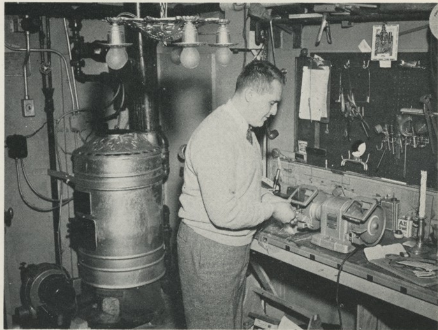
Lang is working on the power grinder in the well equipped workshop, formerly the baggage compartment of the car. Heat for the car is provided by the oil burner in the background.
